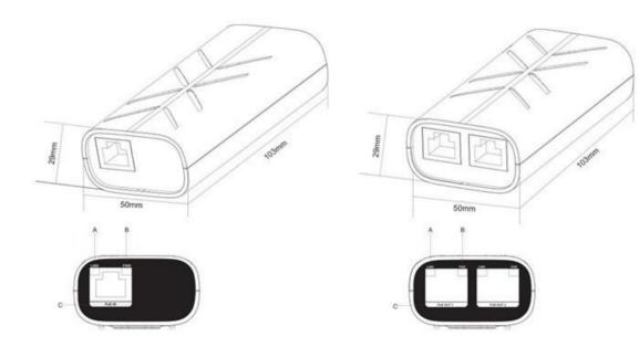
A. Network working indicator B. Power Indicator C. PoE input port
