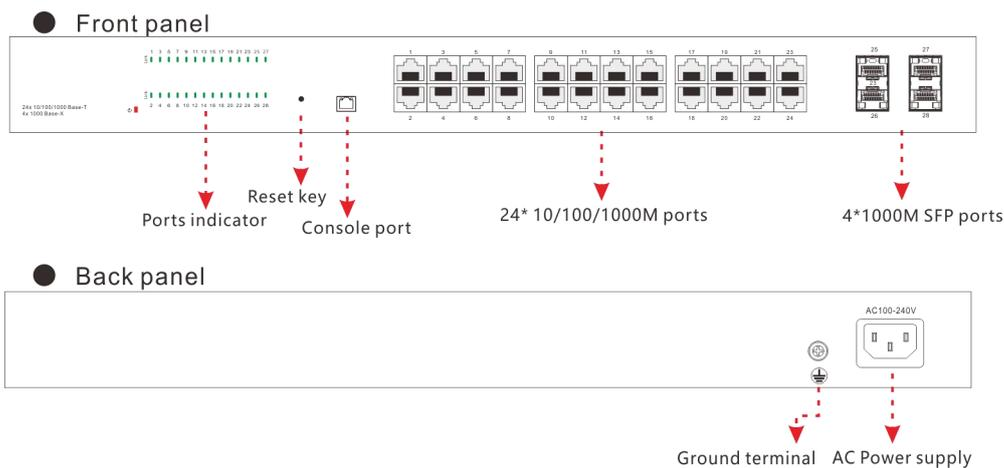
⚠ **Attention 1:** This product must be well grounded against lightning, please use better than 20# cable to connect the grounding terminal and ground.
