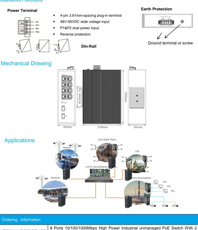
IES7211-8PGE2GF-4BT SFP,1-4Ports support 90W.Din Rail.IEEE802.3af/at/bt
